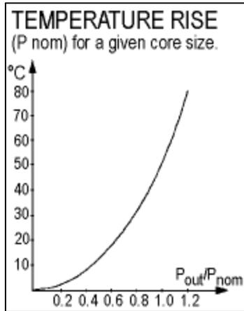
Using a larger core size will reduce the temperature rise. The small core losses will cause the temperature rise to drop drastically when reducing the output power. At half the load, the temperature rise will only be about 25% of the rise at full load.
